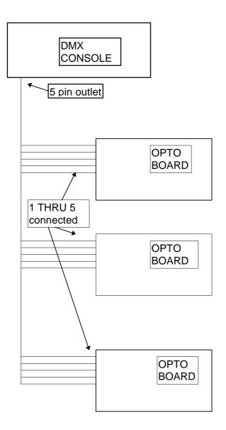
Connect all 5 pins as shown in diagram. Up to 32 isolator boards can be connected to the one desk outlet. Each isolator output will supply up to 32 DMX devices once again. Connecting all 5 pins means the system has compatability with devices that may require talkback lines.
